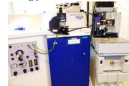
Fig.5 ESI Q-ToF with CapLC
