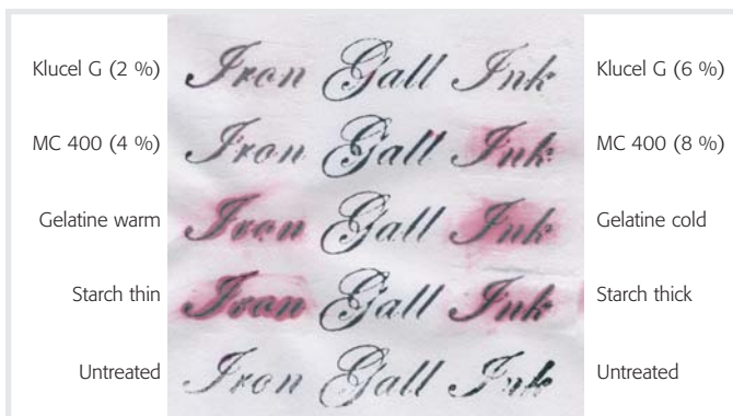
13 Iron(II) migration due to brushing adhesive through repair paper (recto).
