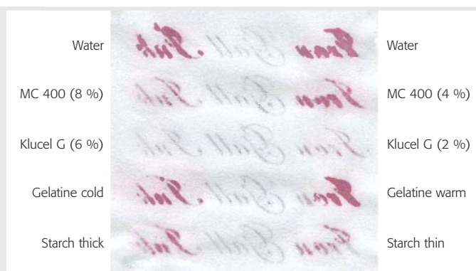
10 Iron(II) migration due to direct application of adhesives (verso).
