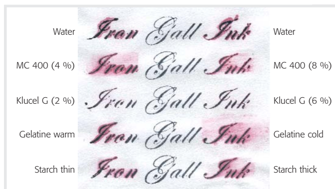
9 Iron(II) migration due to direct application of adhesives, (recto).
