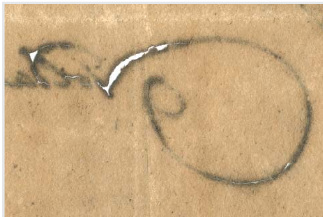
1 Where ink saturated the paper, it is weak and cracks when stress is applied.
