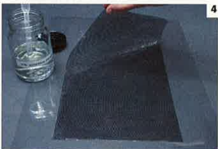
4 Carefully peel away the screen, start at one corner. Be sure not to slide the screen during this operation. Also be careful at the end: when the screen is of the stiff(er) type it will suddenly sweep loose and brush the gelatine away.
