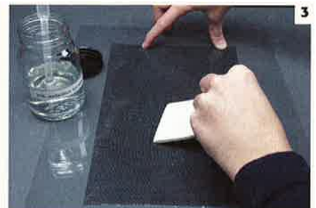
3 Spread the gelatine with the squeegee and even out the gelatine, add more gelatine if necessary, all of the surface of the screen should be filled with gelatine.
