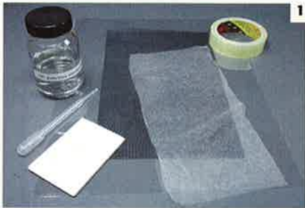
1 Tools and materials for remoistenable tissue. The purpose of the screen is to control the thickness and homogeneity of the gelatine layer.
